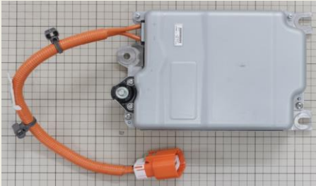
Enclosure and PCB of the 12V DC-DC converter
