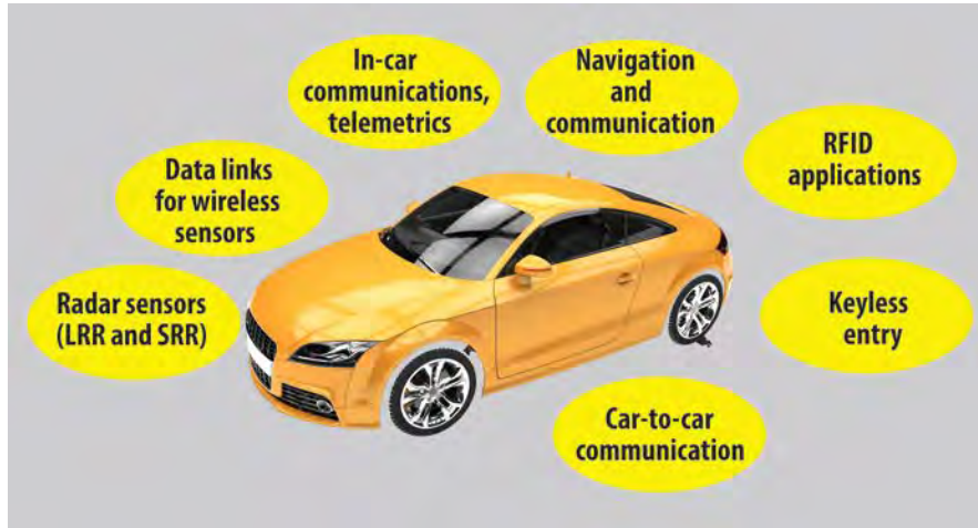
Figure 2. Key elements of advanced automotive RF applications
